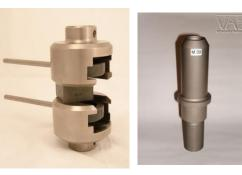
Sample holder for tests with graphite samples.
